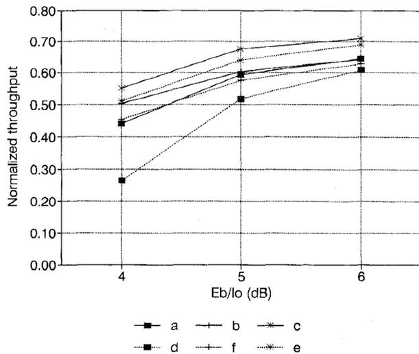
Fig. 8. Normalized throughput for alphabet size.  $f_D T_P = 0.01$ ,  $Y_s = 7.5$  dB. (a) RS (15, 11), (b) RS (31, 23), (c) RS (63, 47), (d) RS (15, 11) with EDA, (e) RS (31, 23) with EDA, and (f) RS (63, 47) with EDA.
