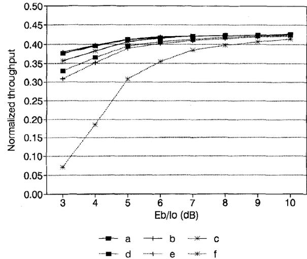
Fig. 4. Normalized throughput of RS (7, 3) code for symbol erasure threshold.  $f_{DT_P} = 0.01$ ,  $M = 8$ . (a)  $Y_s = 3.5$  dB, (b)  $Y_s = 5.5$  dB, (c)  $Y_s = 7.5$  dB, (d)  $Y_s = 3.5$  dB with EDA, (e)  $Y_s = 5.5$  dB with EDA, and (f)  $Y_s = 7.5$  dB with EDA.
