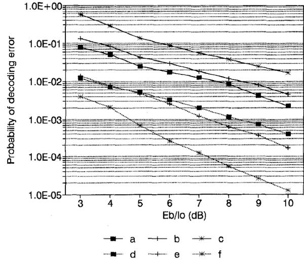
Fig. 3. Probability of undetected error among accepted codewords of RS (7, 3) code for symbol erasure threshold.  $f_{DT_P} = 0.01$ ,  $M = 8$ . (a)  $Y_s = 3.5$  dB, (b)  $Y_s = 5.5$  dB, (c)  $Y_s = 7.5$  dB, (d)  $Y_s = 3.5$  dB with EDA, (e)  $Y_s = 5.5$  dB with EDA, and (f)  $Y_s = 7.5$  dB with EDA.
