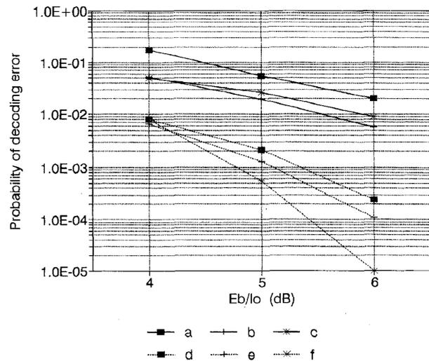
Fig. 7. Probability of undetected error among accepted codewords for alphabet size.  $f_D T_P = 0.01$ ,  $Y_s = 7.5$  dB. (a) RS (15, 11), (b) RS (31, 23), (c) RS (63, 47), (d) RS (15, 11) with EDA, (e) RS (31, 23) with EDA, and (f) RS (63, 47) with EDA.
