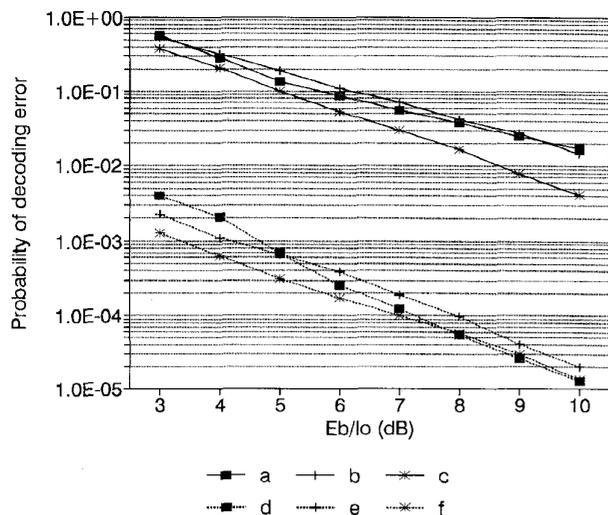
Fig. 5. Probability of undetected error among accepted codewords of RS (7, 3) code for normalized power control interval.  $M = 8$ ,  $Y_s = 7.5$  dB. (a)  $f_D T_P = 0.01$ , (b)  $f_D T_P = 0.02$ , (c)  $f_D T_P = 0.05$ , (d)  $f_D T_P = 0.01$  with EDA, (e)  $f_D T_P = 0.02$  with EDA, and (f)  $f_D T_P = 0.05$  with EDA.
