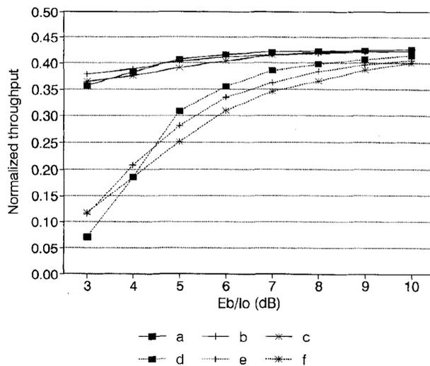
Fig. 6. Normalized throughput of RS (7, 3) code for normalized power control interval.  $M = 8$ ,  $Y_s = 7.5$  dB. (a)  $f_D T_P = 0.01$ , (b)  $f_D T_P = 0.02$ , (c)  $f_D T_P = 0.05$ , (d)  $f_D T_P = 0.01$  with EDA, (e)  $f_D T_P = 0.02$  with EDA, and (f)  $f_D T_P = 0.05$  with EDA.
